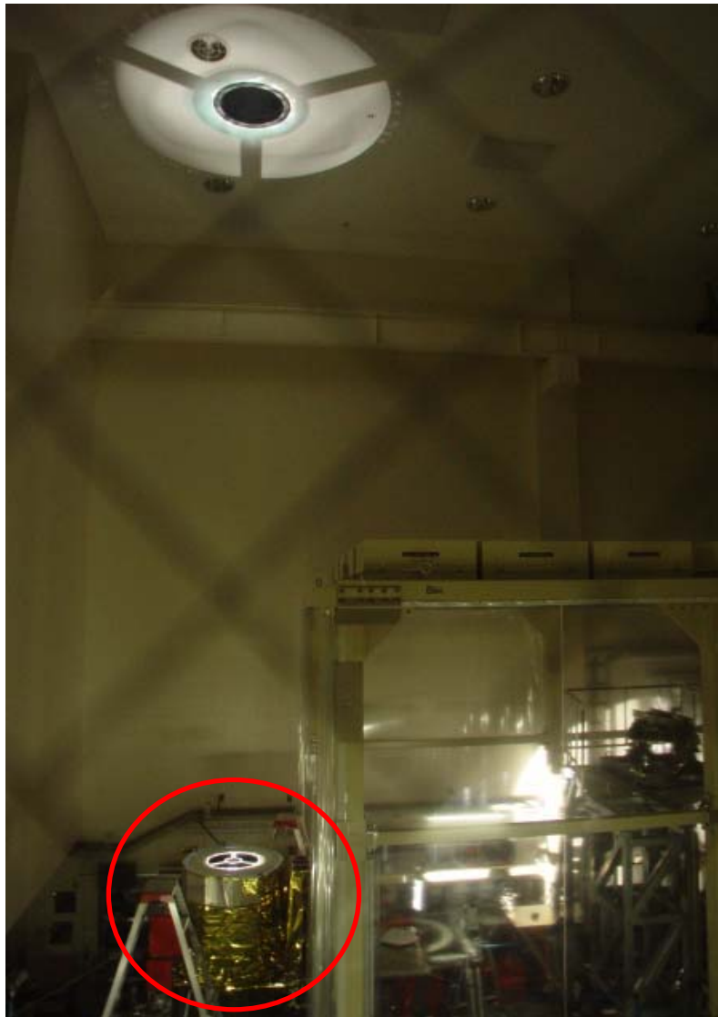
Telescope in clean room illuminated with 50cm sun beam
