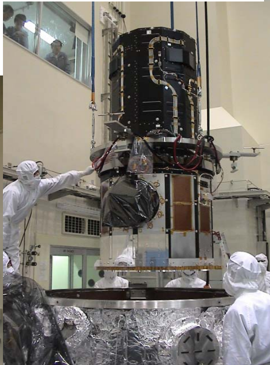
Preparation for Opto-thermal-vacuum test
